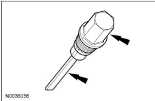
5. Wipe the transmission fluid level indicator clean. Reinstall the transmission fluid level indicator only back into the transmission fluid fill plug hole to check the transmission fluid level.
