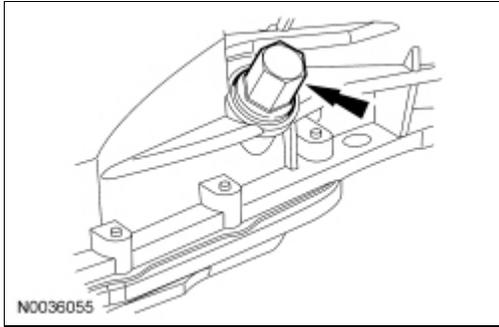
4. Separate the transmission fluid level indicator from the transmission fluid fill plug.
