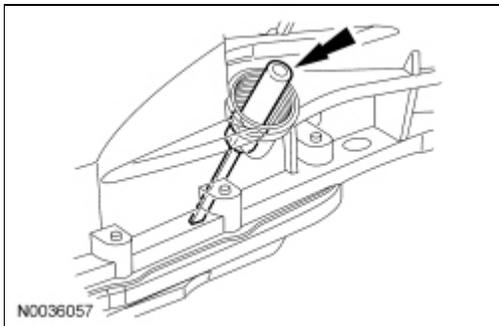
6. **NOTE:** The transmission fluid level indicator has 2 areas for the fluid level, a crosshatched (labeled A) area and a dotted (labeled B) area. Use the dotted (labeled B) area when checking the transmission fluid level. The correct transmission fluid level is at the upper level of the dotted marks on the transmission fluid level indicator.
